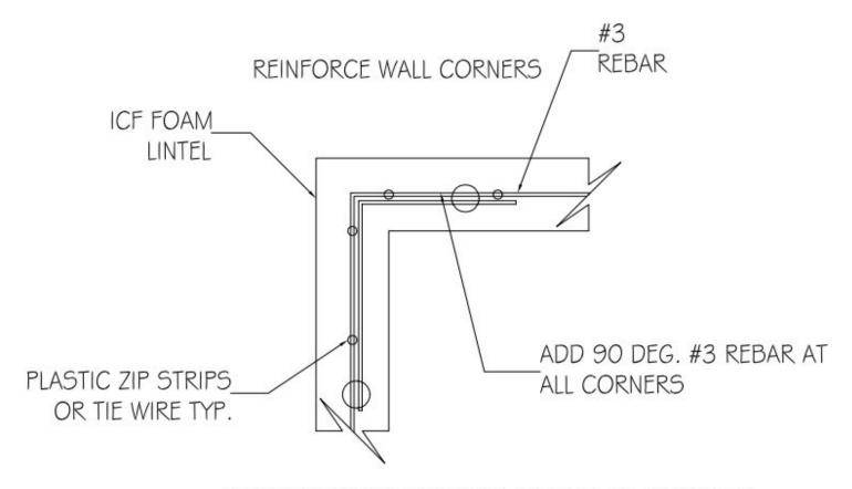
INSIDE/OUTSIDE CORNERS 90 DEG. #3 REBAR TO TIE IN WALLS AT 4' AND 8' HIGH BEAM/LINTELS
