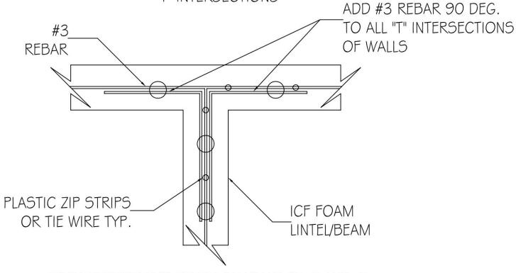
"T" INTERSECTIONS TO TIE IN WALLS AT 4' AND 8' HIGH BEAM/LINTELS
